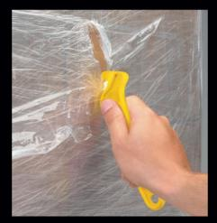
Place thumb on the side grips to firmly guide your cut downward. The tool design and ultra sharp blade maintain the optimum cutting angle for cutting shrink wrap.
